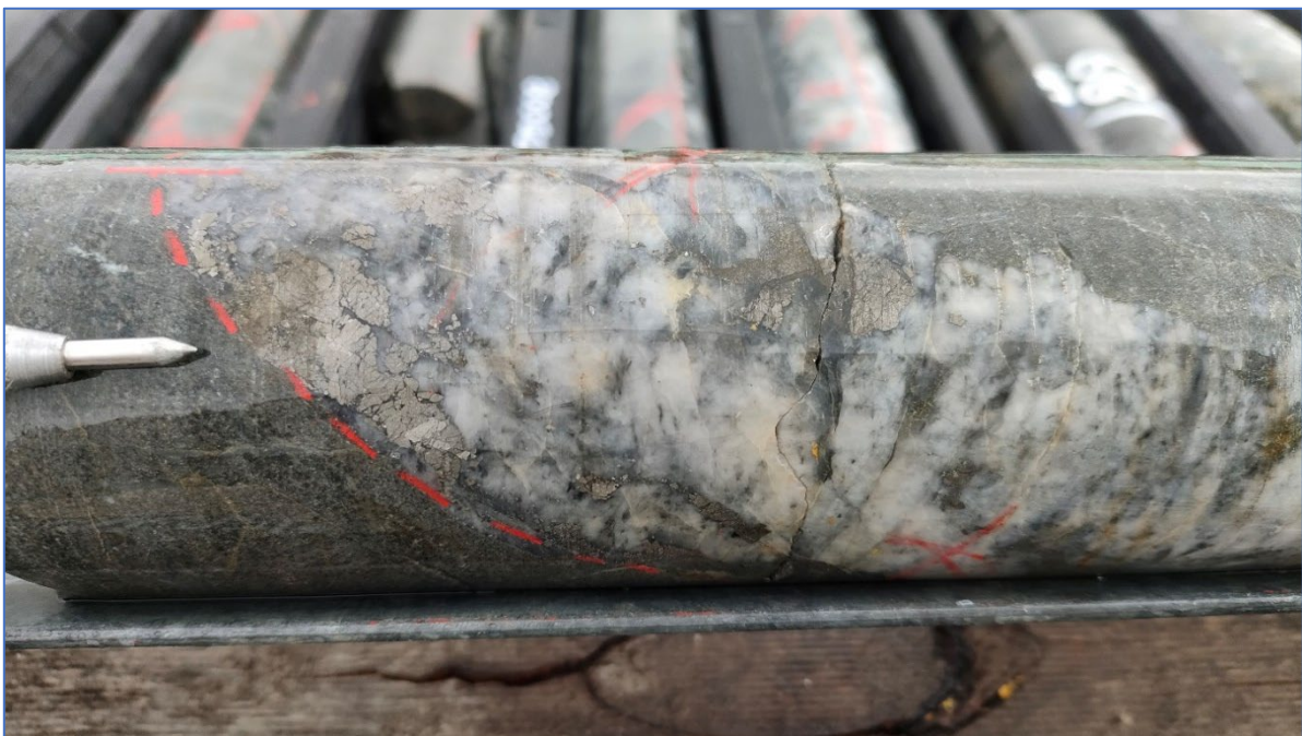
Figure 4: Close-up of TFDD008 core at 93.5m - grey quartz vein with coarse arsenopyrite
