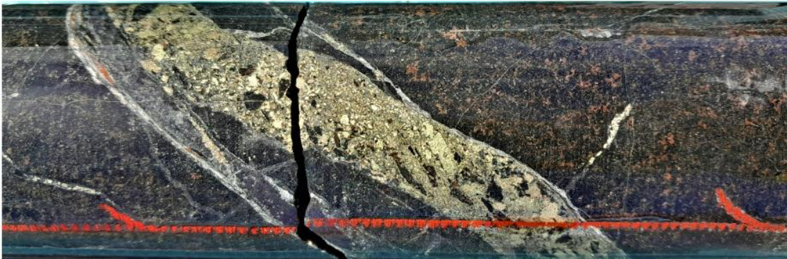
Figure 5: HWDD07 1350.4m Chalcopryite-Pyrite-Quartz vein in mafic intrusive.
