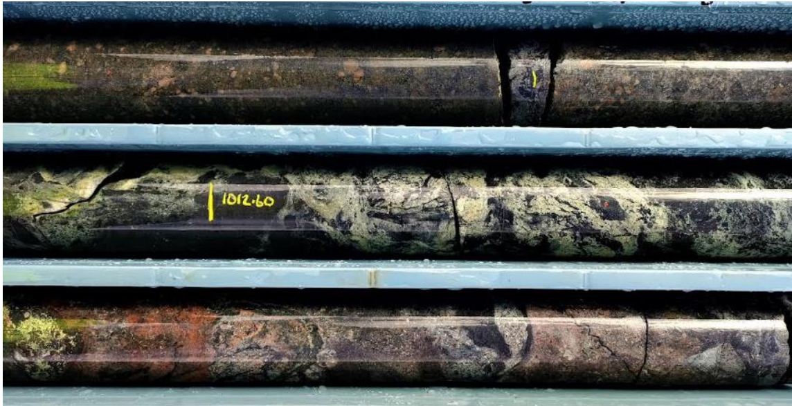
Figure 8: Chalcopyrite encountered in HWDD08 at 1,012m.
