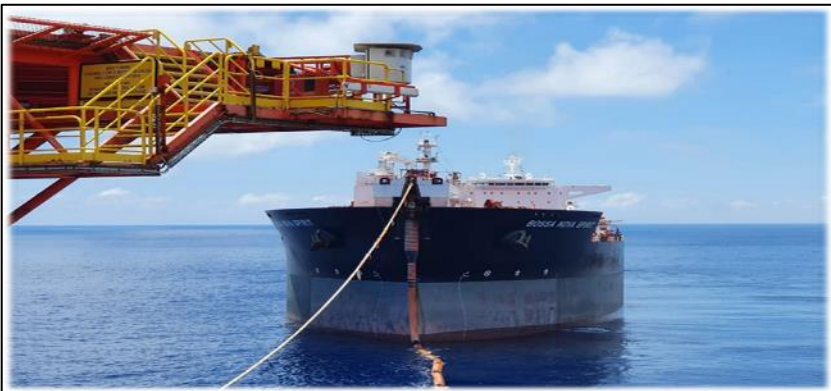
Shuttle Tanker (Shell) Bossa-Nova performing Offloading operation
