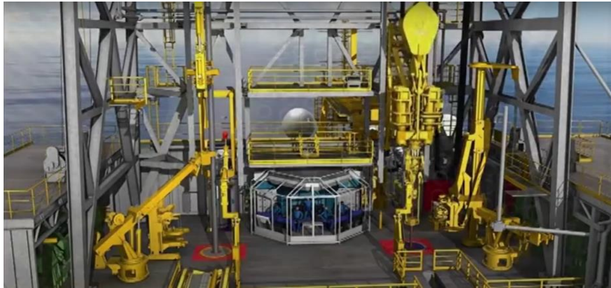
Clip riser connected without manual handling – fast and safe BOP running
