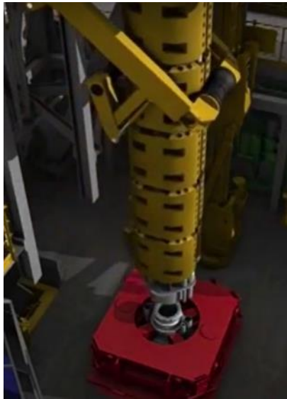
Clip riser connected without manual handling – fast and safe BOP running
