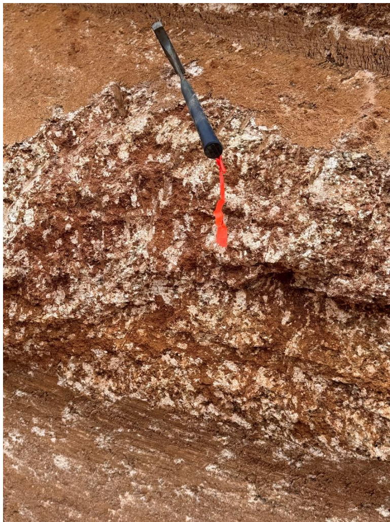
In-situ clay-rich saprolite at Area B
