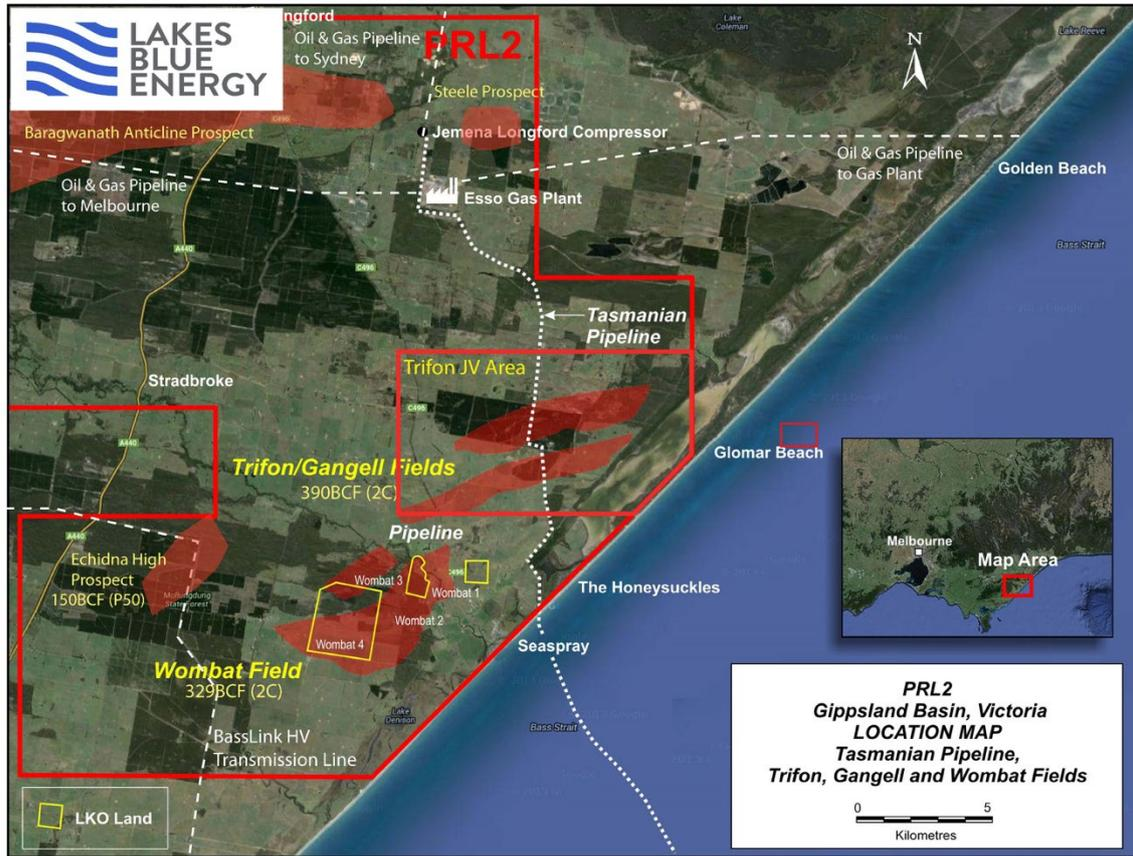
The Company envisages an integrated approach to development of the Wombat and Trifon-Gangell Gas Fields. Sales gas production would initially be from the Wombat Gas Field with the Trifon-Gangell Gas Field developed to support steady gas sales over a 20-year period. On this basis, the estimated conventional sales gas potential of the fields is at least 20 PJ/a.
