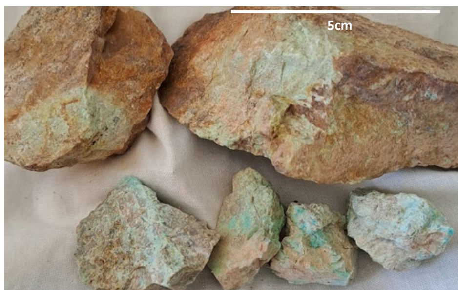
Figure 2: 0.7% Cu returned from pervasive Cu oxide and clasts within hydrothermal rhyolite breccia (Sample 3862)
