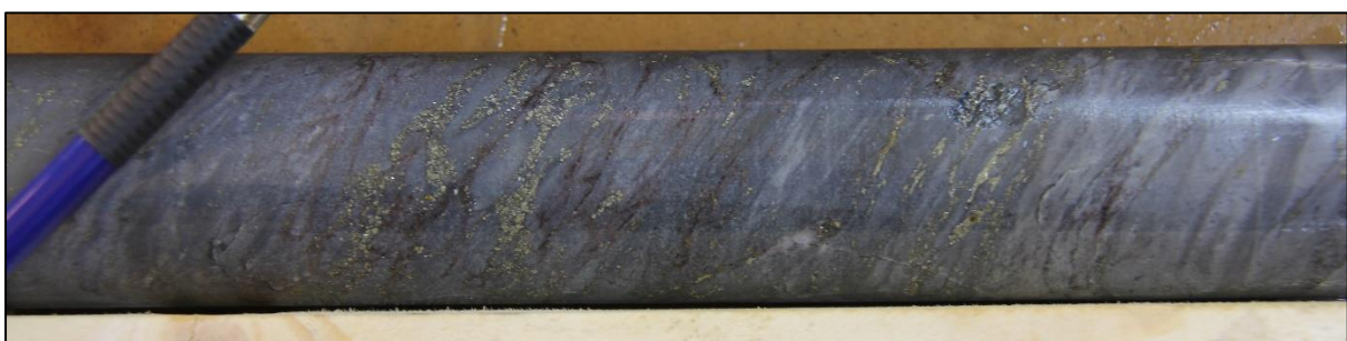
Figure 2. Pyrrhotite, pyrite, and sphalerite in intensely-altered felsic volcano-sedimentary rock. NOR17001, 46.5m.
