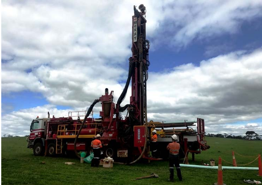
Figure 1 – RC Drill on site at the Garard Ni-Co prospect
