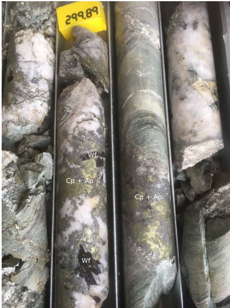
Figure 3 – High grade vein mineralization within SVS (CRD009 from 229.00 m – 302.00 m, only part of section visible. Wf = wolframite, Cp = chalcopyrite, Ap = arsenopyrite.
