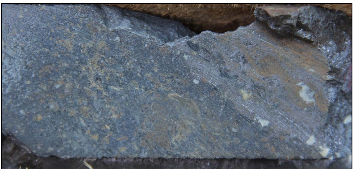
Figure 10. High-grade disseminated to semi-massive sphalerite-galena mineralisation in altered tuff, SHDD001, 229m (NQ core diameter 47.6mm)
