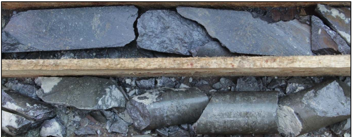
Figure 9. High-grade disseminated to massive sphalerite-galena mineralisation in altered tuff, SHDD001, 229m (NQ core diameter 47.6mm)
