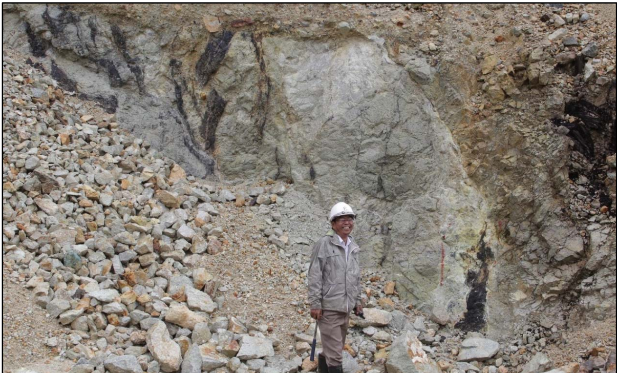
Figure 6. Mineralised face in the Chinaman open pit at Bawdwin. High-grade mineralised zones (black) occur in altered tuff with disseminated sulphide. Channel CH011 across this face returned 8m at 5.1% Pb, 12.1% Zn and 129 g/t Ag. Note the old stope at right.
