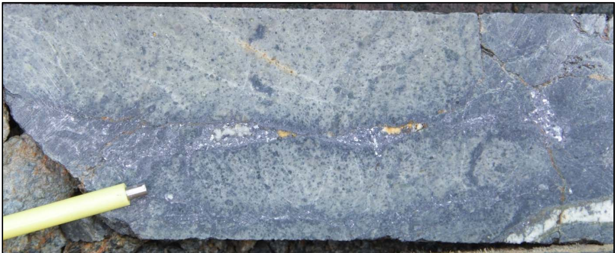
Figure 12. Stockwork and disseminated galena-sphalerite mineralisation in altered porphyry, SHDD001, 47.6m (HQ core diameter 63.5mm)
