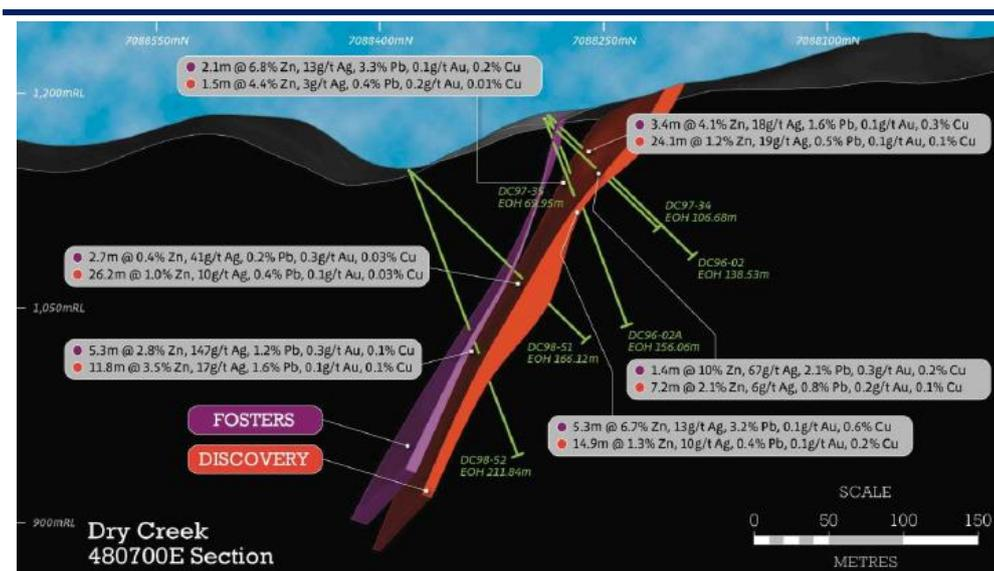
Figure 8. DC cross section at 480700E, looking East through lenses
