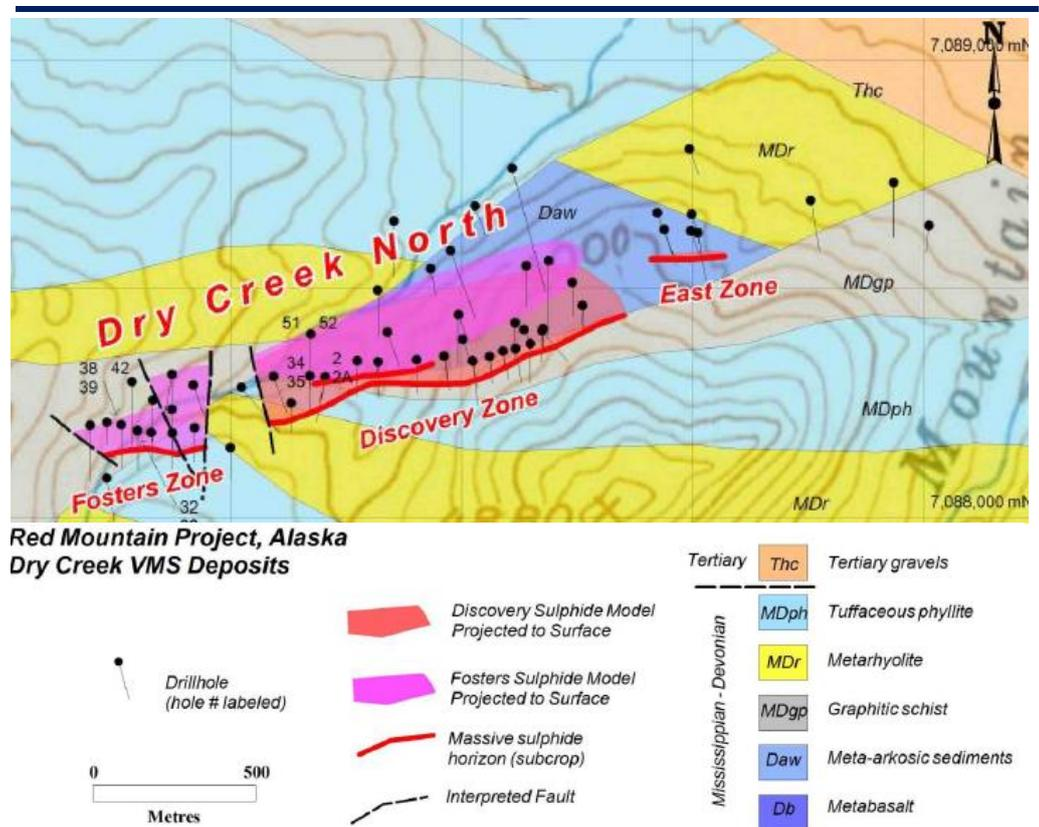
Figure 7. Dry Creek geology and lenses projected to surface
