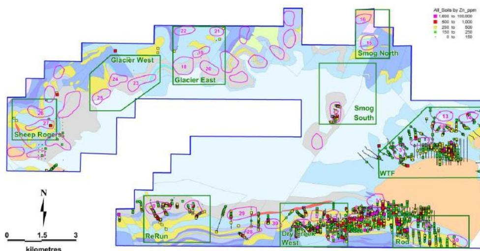
Figure 12. Zinc geochemistry on geology and conductors
