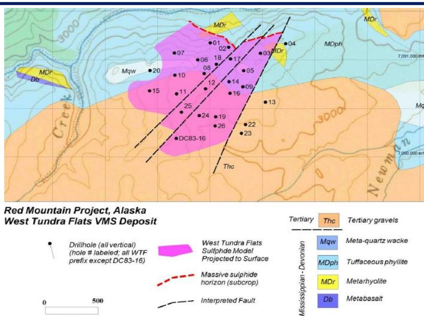
Figure 9. WTF mineralisation projected to surface with geology
