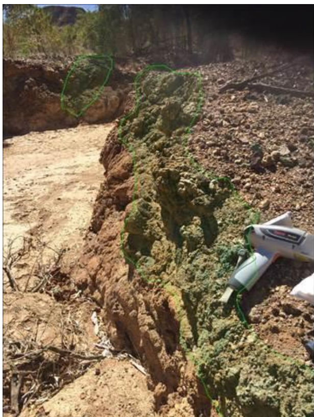
Figure 2: WM001 (1) within resource area, NitonXRF values of 0.17% Co and 16.42% Cu .
