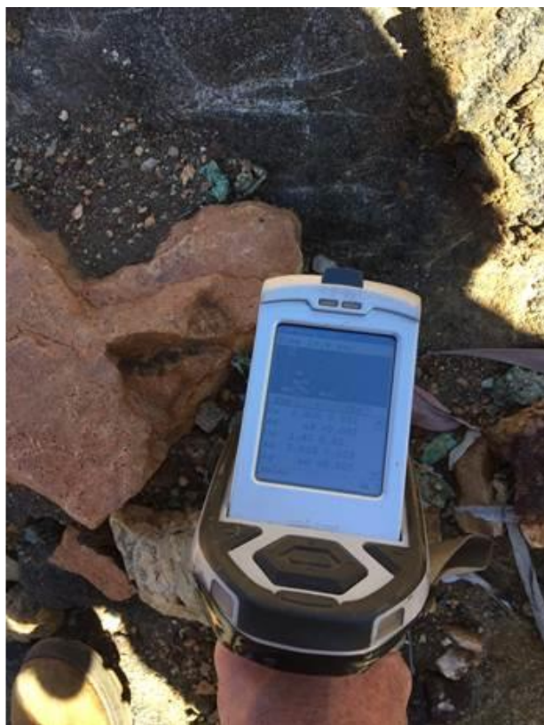
Figure 3: WM002 (2) within resource area, NitonXRF values of 1.28% Co and 1.18% Cu , and 0.8% Co and 1.42% Cu respectively.
