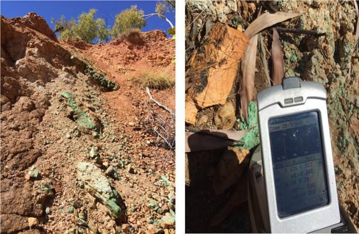
Figure 6: WM006 (6) within resource area, NitonXRF values of 0.126% Co and 24.38% Cu .
