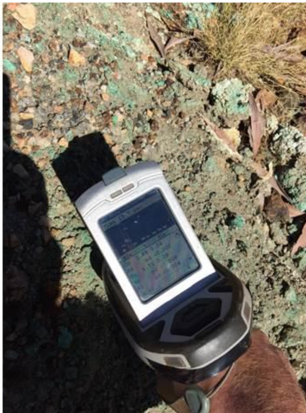
Figure 5: WM005 (5) within resource area, NitonXRF values of 1.88% Co and 5.71% Cu .
