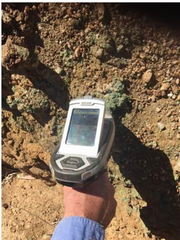
Figure 2: WM001 (1) within resource area, NitonXRF values of 0.17% Co and 16.42% Cu .
