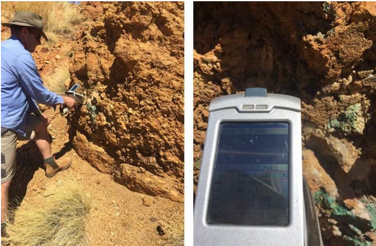
Figure 8: Southern extension showing NitonXRF values of 0.94% Co and 7.45% Cu .
