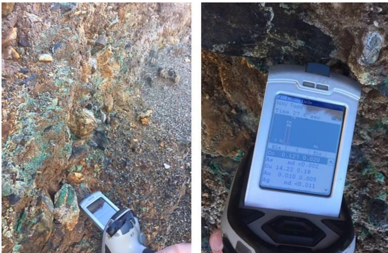
Figure 11: Sample from Rosebud showing NitonXRF values of 0.127% Co and 14.22% Cu .
