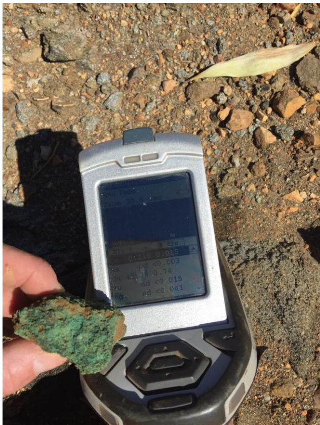
Figure 4: WM003 (3) within resource area, NitonXRF values of 0.21% Co and 45.38% Cu .
