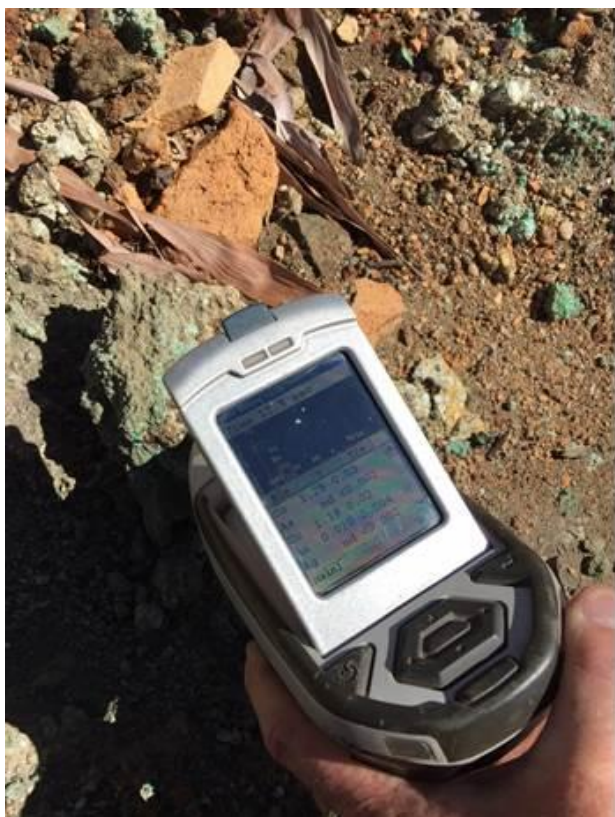
Figure 3: WM002 (2) within resource area, NitonXRF values of 1.28% Co and 1.18% Cu , and 0.8% Co and 1.42% Cu respectively.
