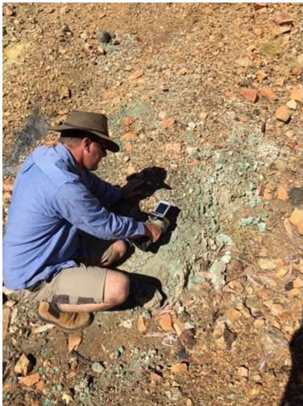
Figure 5: WM005 (5) within resource area, NitonXRF values of 1.88% Co and 5.71% Cu .
