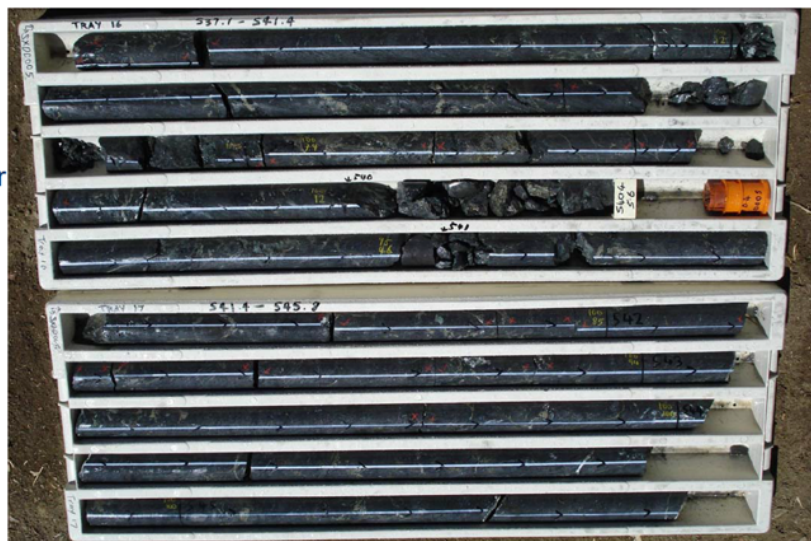
Figure 8: Core photos from SXDD005 537-546m showing Graphite Schist
