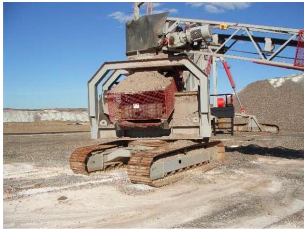
*Figure 8 - Crawler-mounted radial stacker conveyor*
