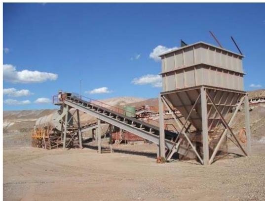
*Figure 2 - Bin discharge conveyor*
