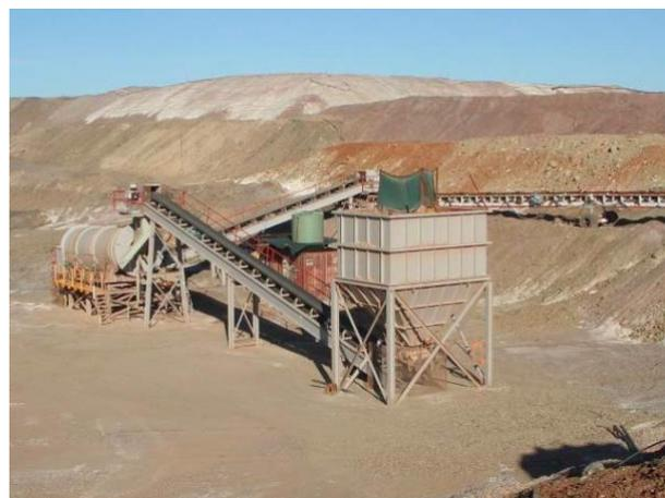
*Figure 3 - Bin discharge conveyor*
