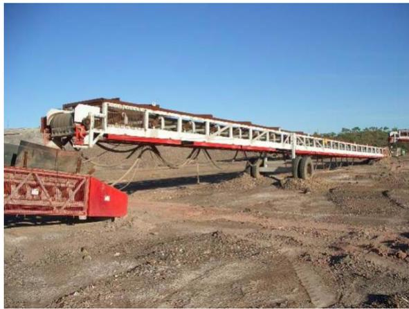
*Figure 5 – Agglomerator discharge conveyor*
