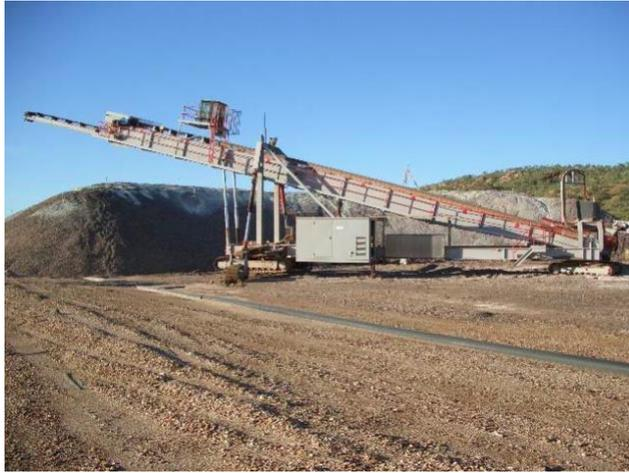
*Figure 7 - Stacker infeed conveyor*
