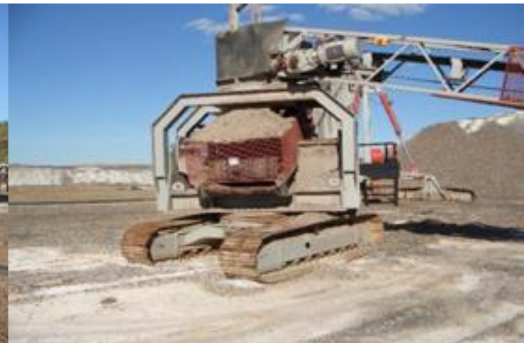
Figure 8 - Crawler-mounted radial stacker conveyor
