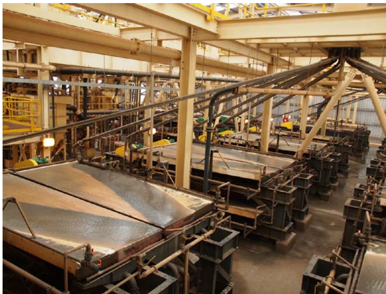
Figure 5.3 Wet tabling machine area
