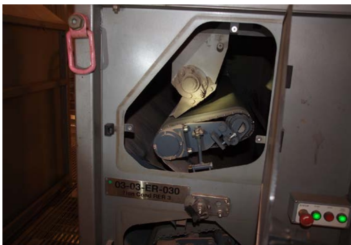
Figure 5.6 Rare earth roll magnetic separator (RER)
