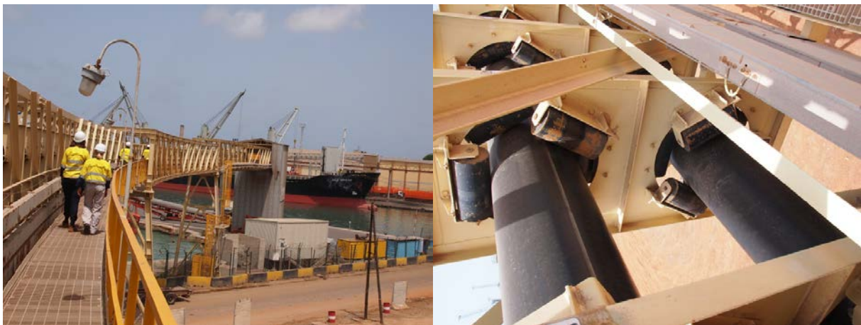
Figure 8.6 Tube conveyor
