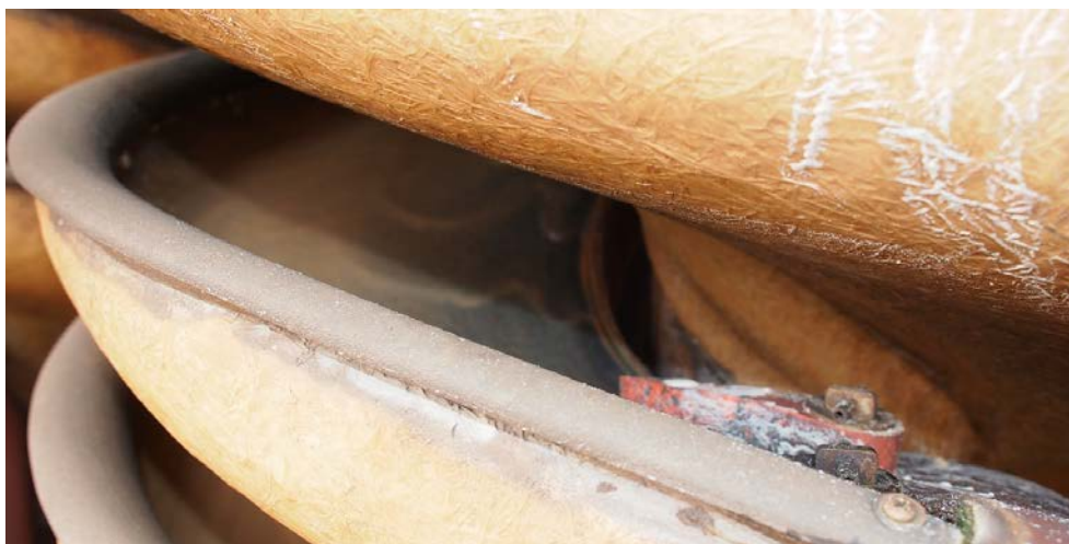
Figure 4.2 Non-efficient sand flow in the rougher spiral
