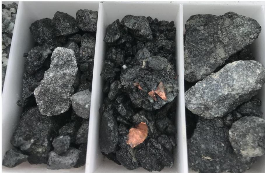
**Figure 4 – Native copper in drill chips from QRC 150 between 114-115 metres.**
