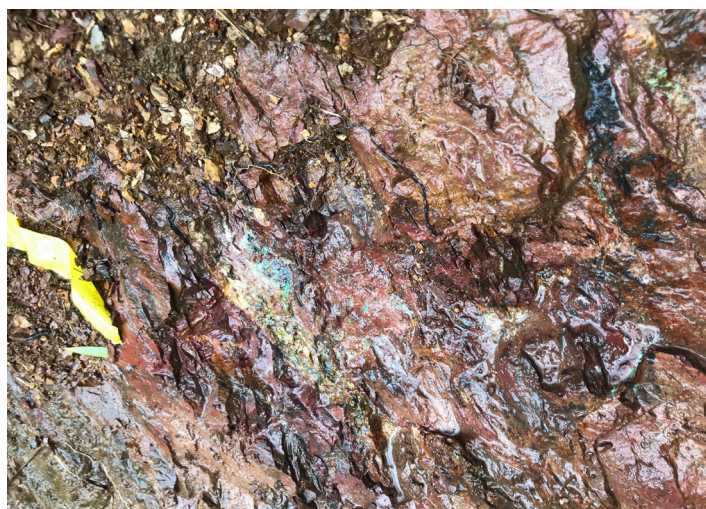
Figure 2: Silicified hematitic mudstone with malachite.
