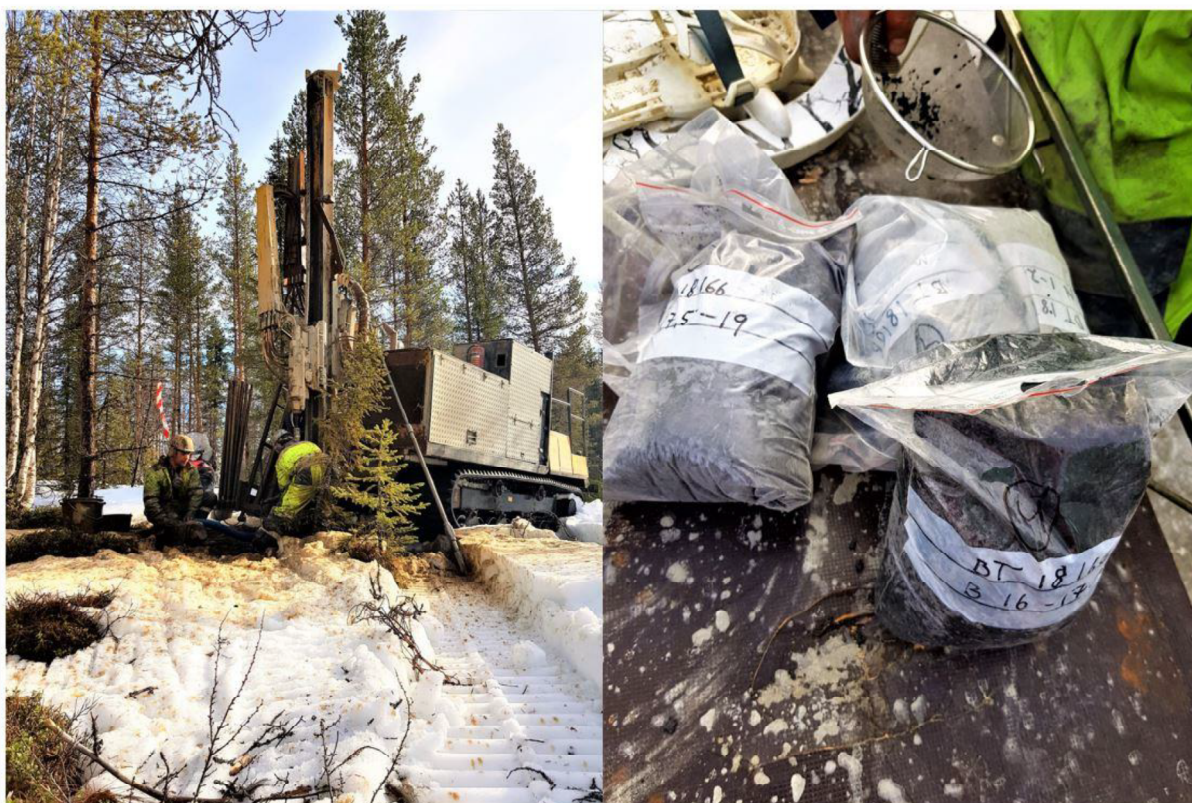
Figure 3: Photos from the recently completed bottom-till geochemical drilling at the Norrliden Project, Sweden.
