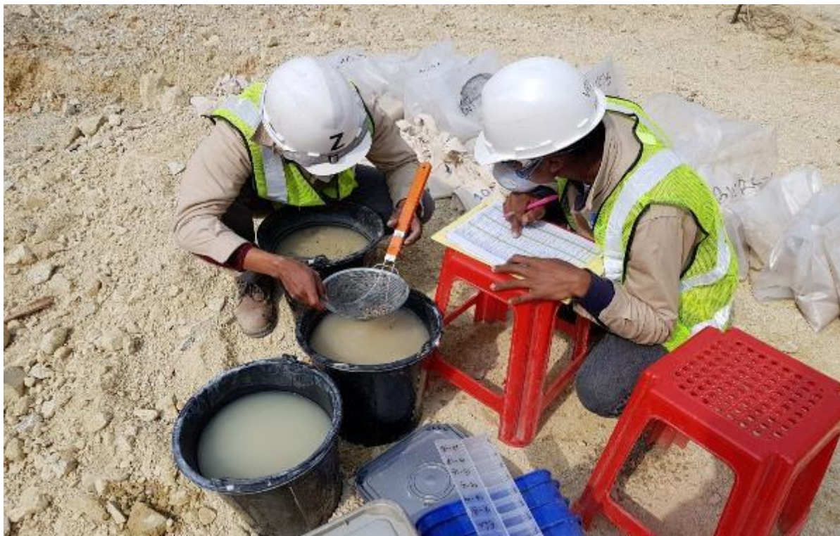
RC Sample logging at Bawdwin, March 2018. Image: Valentis Services
