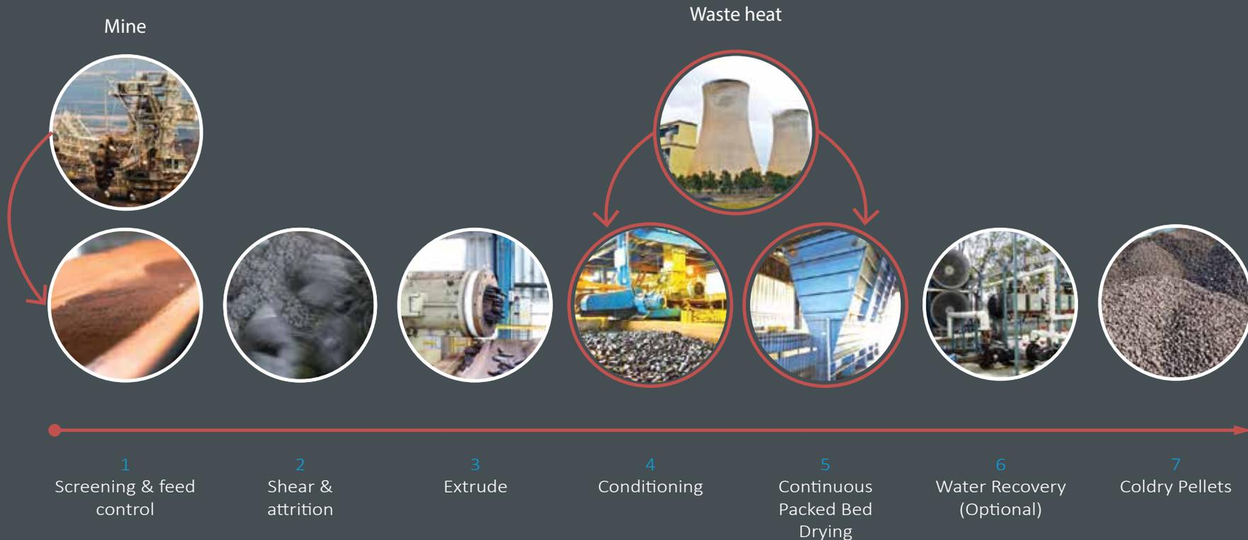
**1** Primary processing begins when brown coal is mined and delivered to the Coldry plant where it is milled and screened to achieve a consistent size.
