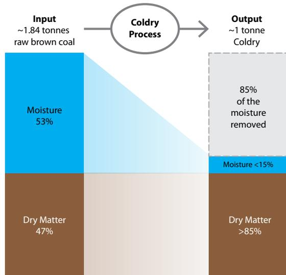
The Coldry process specifically targets the removal of moisture, leaving the dry matter in place.
