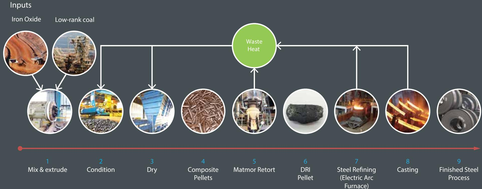
**1** Iron ore fines are combined in a specific ratio with lignite, then processed through the Coldry Process, beginning with shearing and extrusion.
