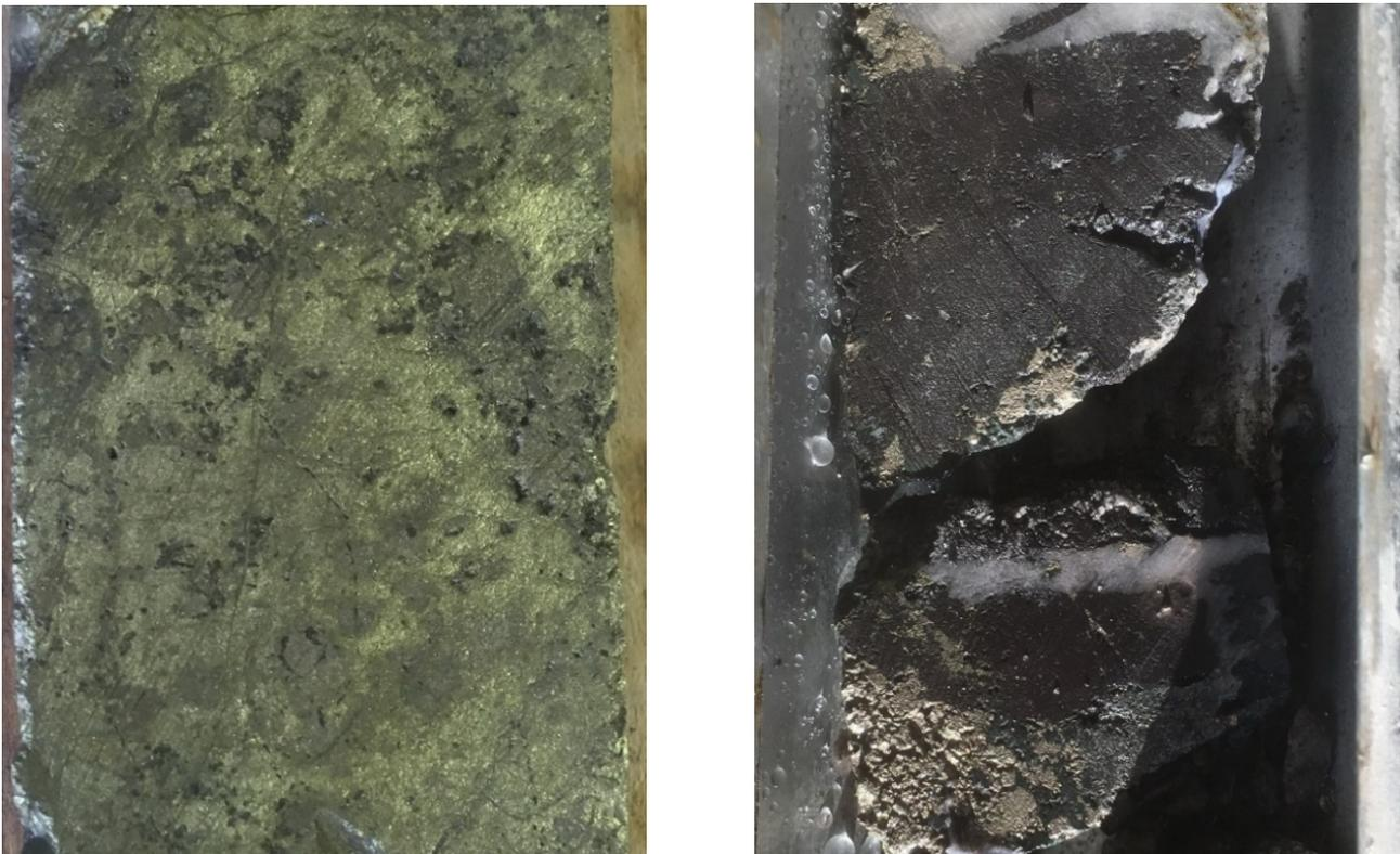
Figure 2 – Core photographs of exceptionally high grade 'Including' intercepts; L – CRD018: 358.72 m, solid chalcopyrite with wolframite (interval contains 10.73% Cu and 3.42% WO<sub>3</sub>), R - CRD019: 510.95 m, solid wolframite (interval contains 8.58% WO<sub>3</sub>)
