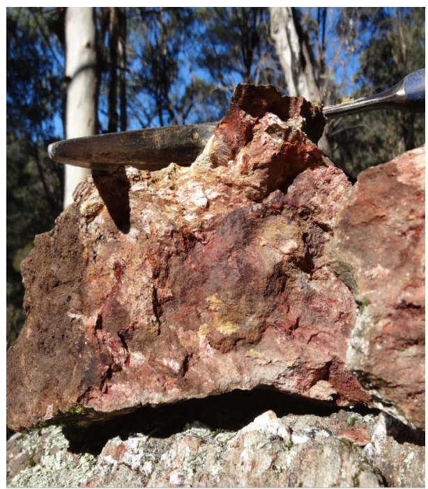
Photograph 3. Close up – sample broken from outcrop shown in Photograph 2. Sample is silicified sandstone showing abundant iron staining after disseminated sulphide with clots of limonite and minor quartz veining. This is an example of the mineralisation style within the Fairleys Shear Zone. (Geology pick for scale)
