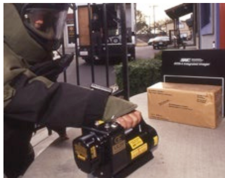
Above – Current bomb disposal X-ray imaging technique
