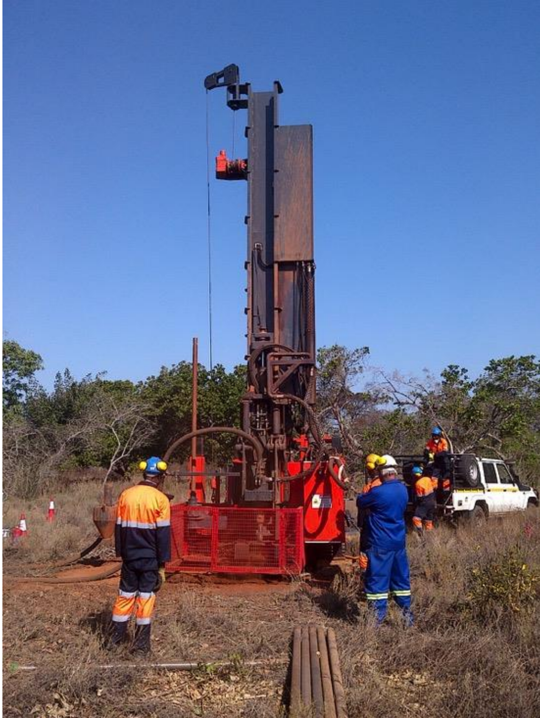
Figure 2: Aircore drill rig operation at Koko Masava
