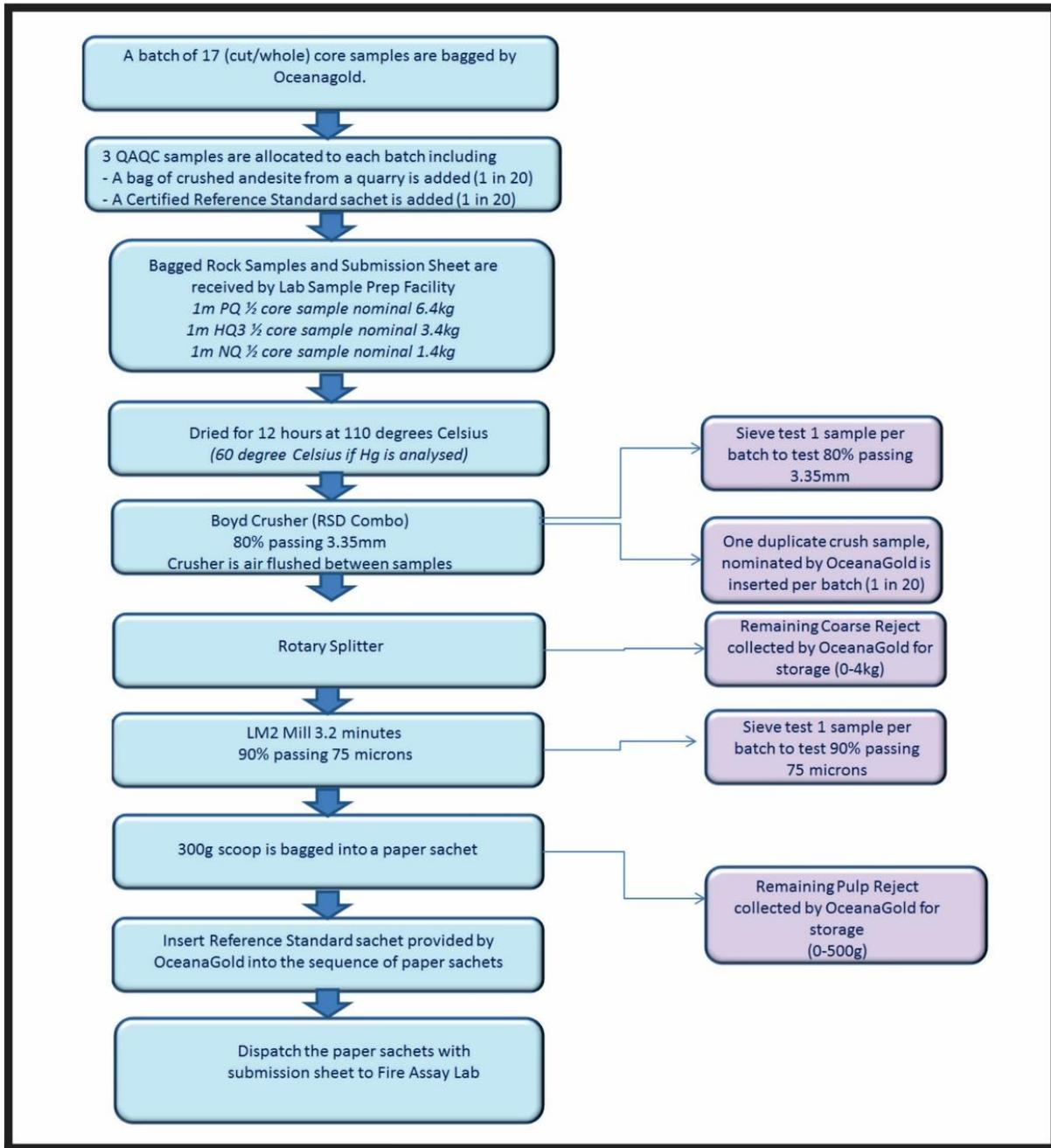
Figure 11.1: Sample Preparation Flow Sheet SGS, Waihi
