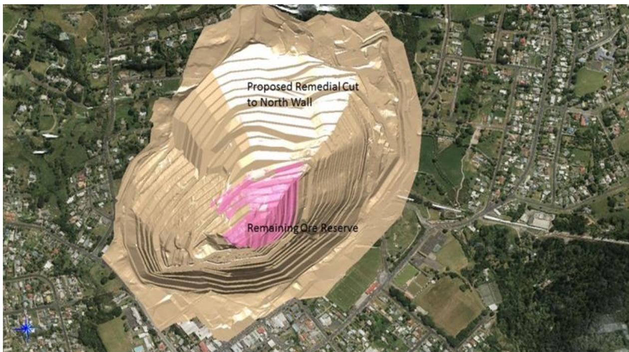
**Figure 15.1: Open Pit Mineral Reserve Limits and Stability Cutback**
