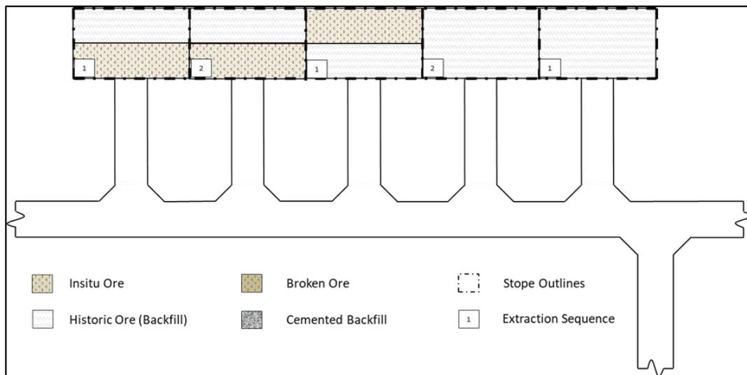
**Figure 14.20: Side Ring Mining Method - Plan**
