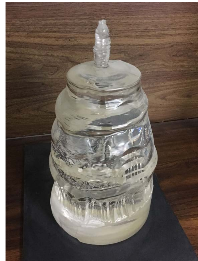
Sapphire Crystal Boule made from Polar HPA
