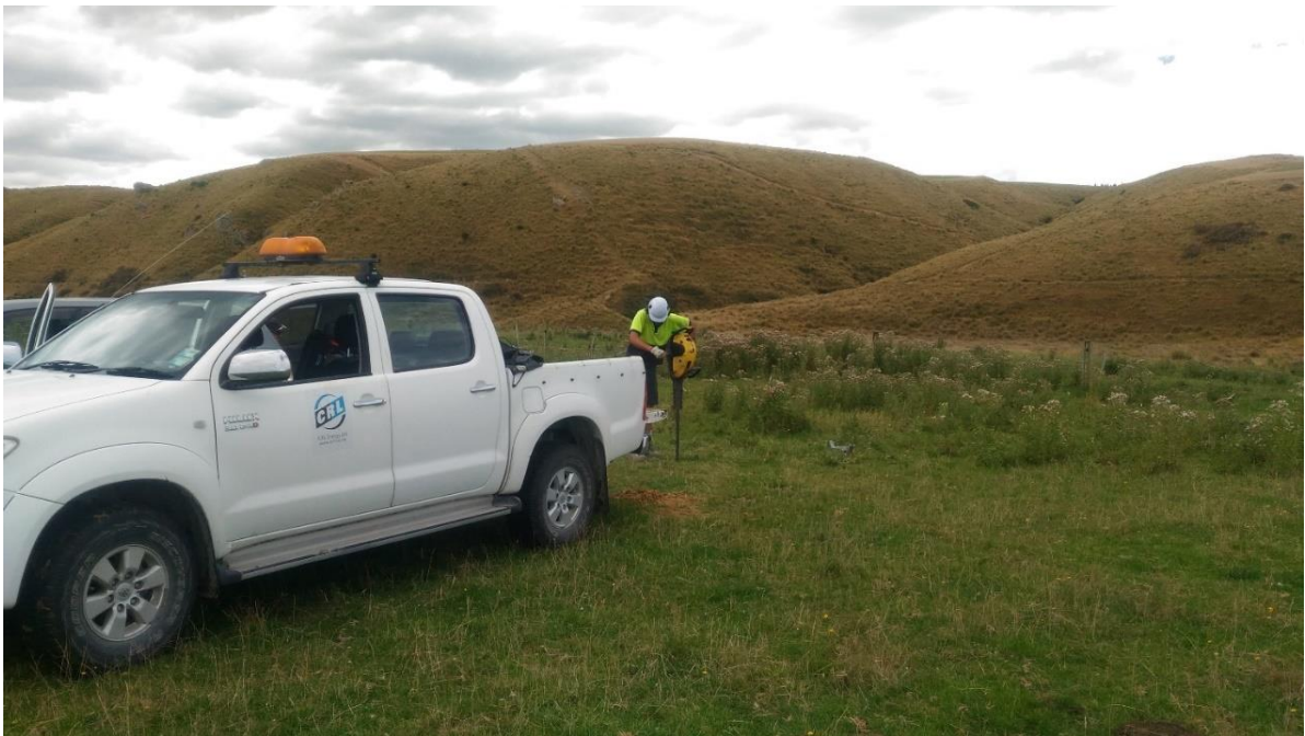
Figure 9 - September 2018 Fieldwork - soil sampling with man-portable drill
