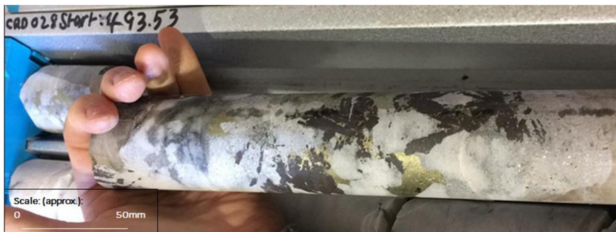
Figure 4 - Well-developed wolframite and chalcopyrite, in interval 493.16-493.91m, CRD028
