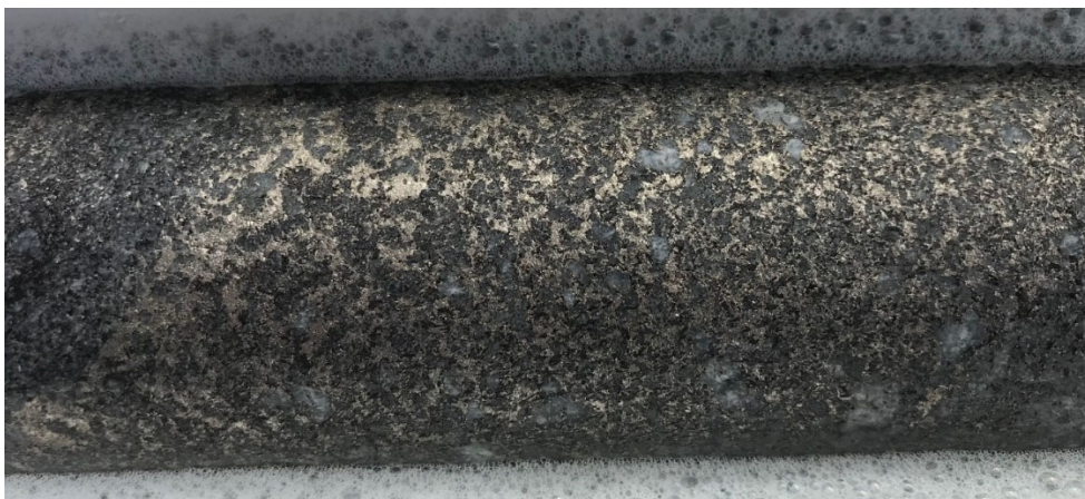
Figure 10 – Massive sulphide mineralisation from hole QDD0004, length 15cm, approximately 214 metres depth downhole
