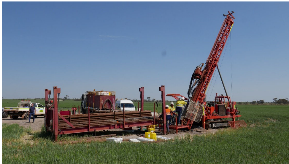
Figure 9 – Diamond drill rig at the Wyatt's prospect.
