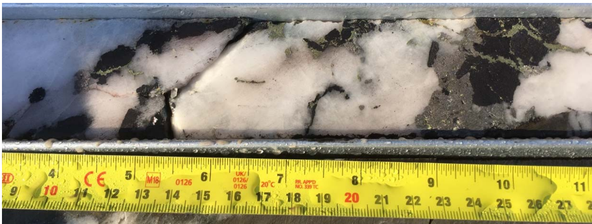
Figure 3 – CRD023: 651m – coarse blocky wolframite in quartz veins
