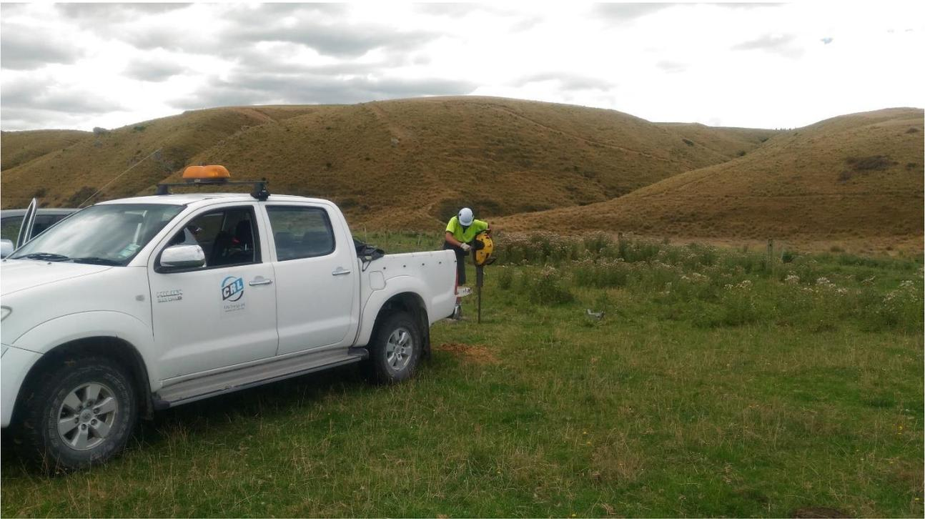
Figure 1 – September 2018 Fieldwork -soil sampling with man-portable drill
