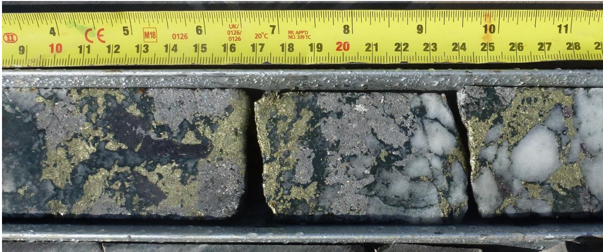
Figure 5– CRD024: 589.5m –wolframite and chalcopyrite in quartz veins
