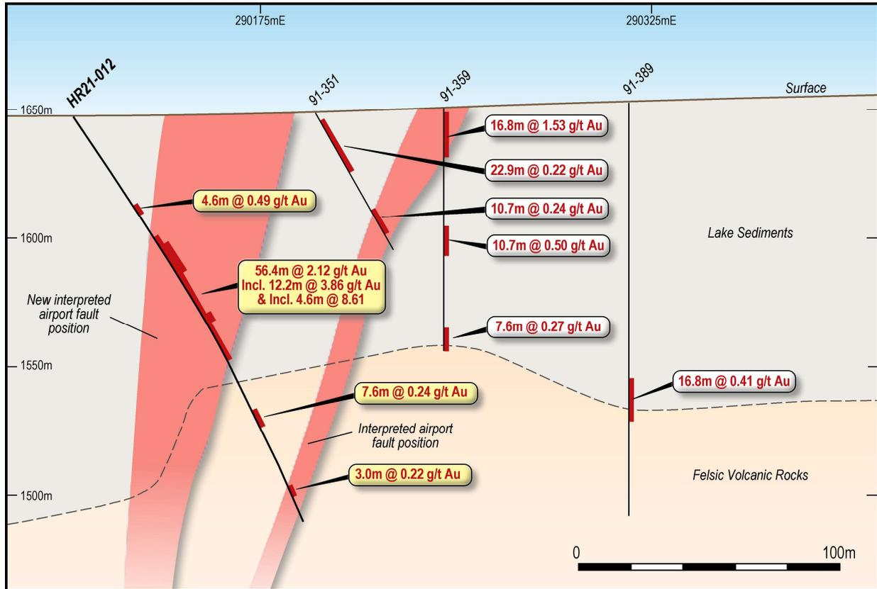
**Figure 2:** Cross section view (see Figure 1 for location) highlighting the drilling results from hole HR21-012 relative to the surrounding historical drilling information.
