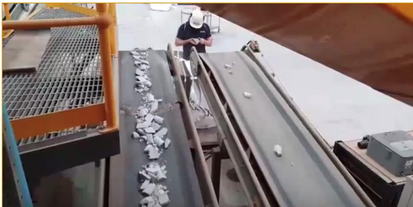
Photo 2. Korbels Drill Core in progress on TOMRA's XRT Ore Sorter
