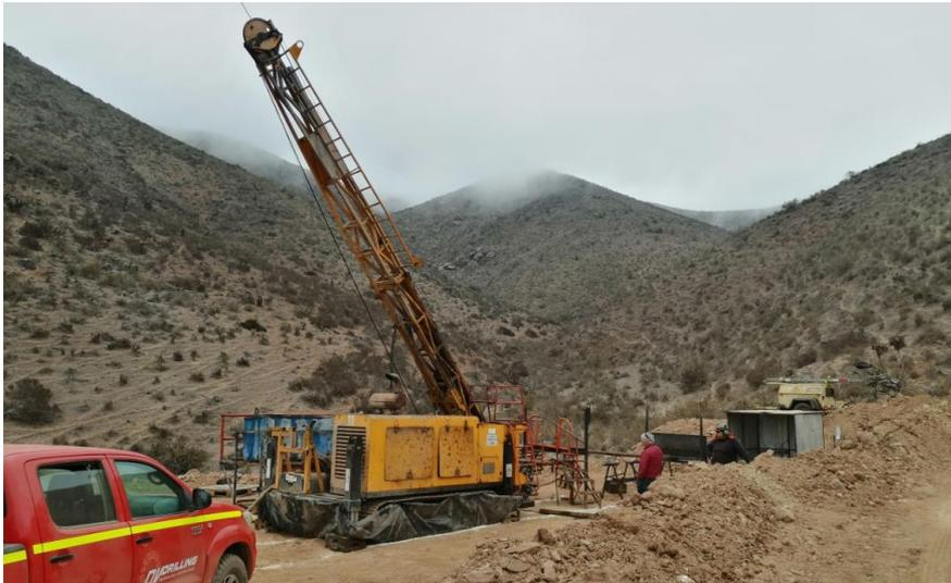
*Diamond rig at previously drilled hole ES-001. 18m at 0.2% Cu aggregated in first 144m. Proposed new holes to be drilled in Valley behind rig. Rig is only 600m from a public road.*
