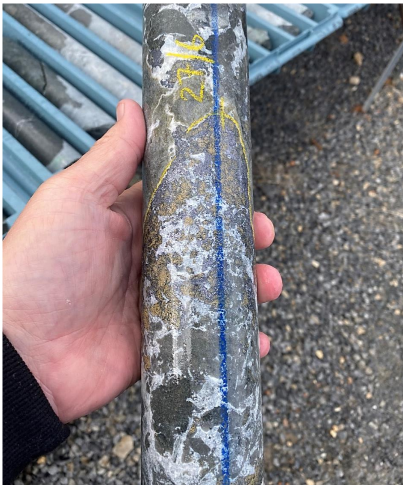
Figure 5: Straw-yellow sphalerite (zinc) and grey galena (lead) mineralisation in quartz + carbonate vein at approximately 213m down hole in GDD003.
