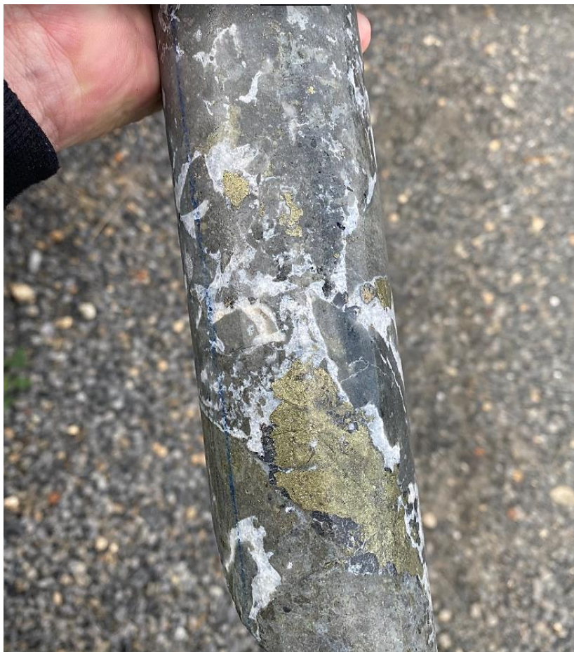
Figure 4: Chalcopyrite (copper) mineralisation at approximately 215m down hole in GDD003.
