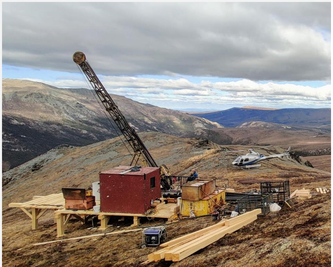
**Figure 1:** Diamond rig set-up to drill hole DC21-97 at the Dry Creek VMS deposit.
