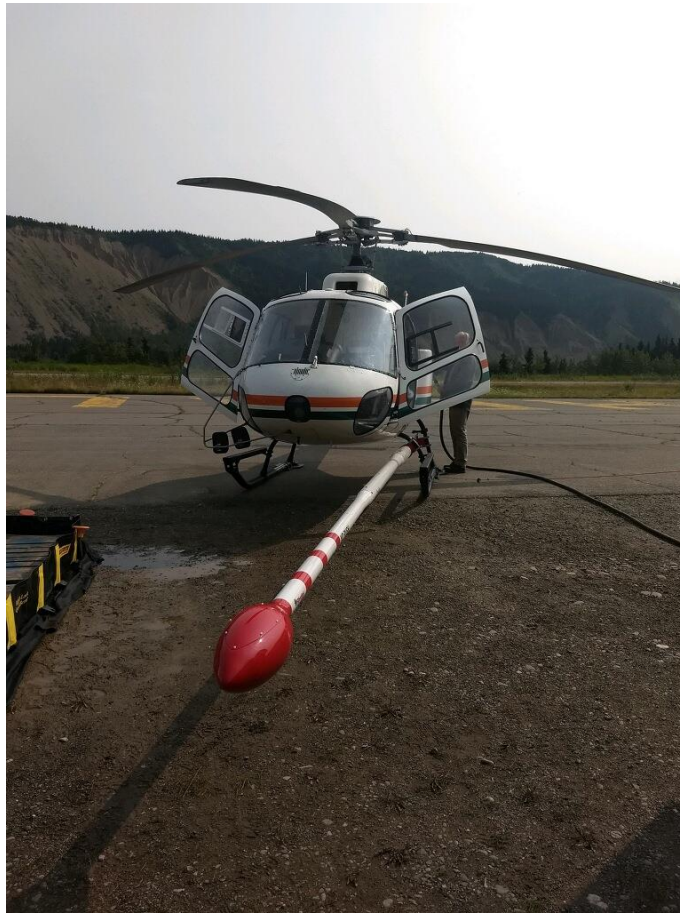
Figure 3: Photo of the helicopter with the nose stinger mounted magnetic sensor.
