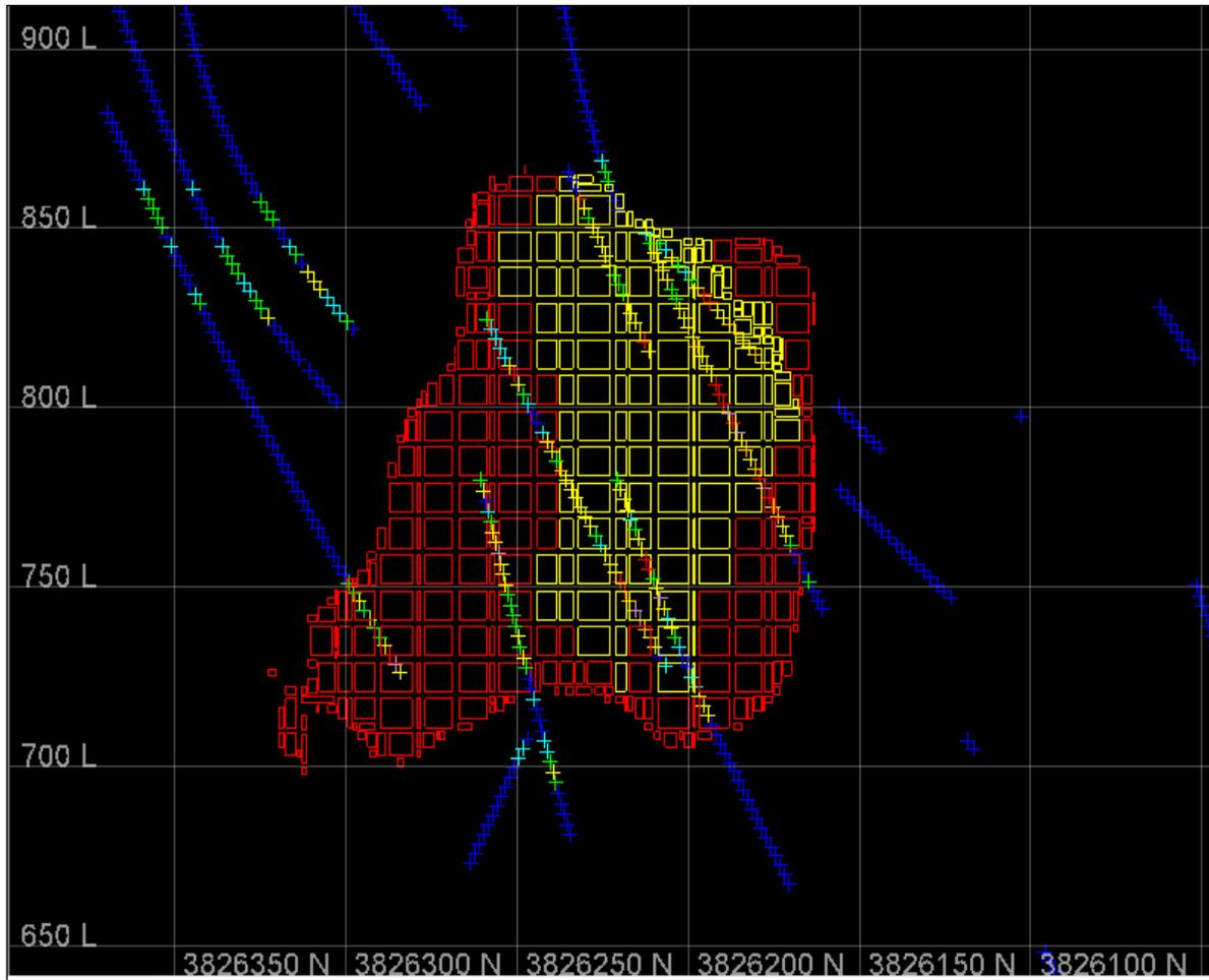
Source: OceanaGold, 2022 Figure 14-27: Representative Cross Section 543,790mE looking E - Showing Resource Classification (Yellow -Indicated / Red - Inferred)
