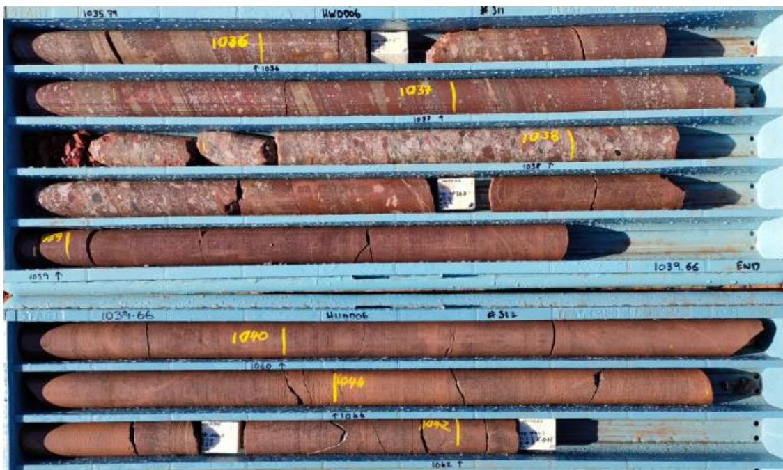
Figure 2: Drill core from HWDD06 (1035.79 – 1042.10m) showing the transition from a basal conglomerate of the Pandurra formation (~1,038.4m) to a weathered mafic intrusive.
