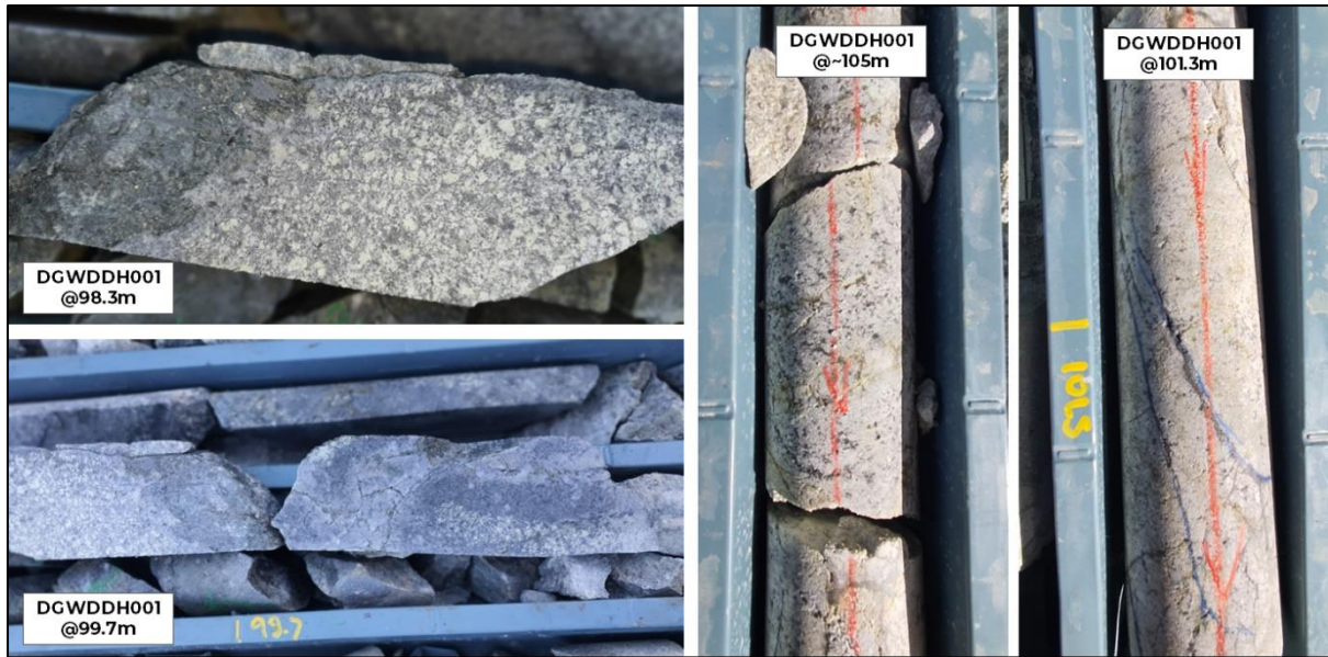
Figure 4: Porphyry intersected in DGWDDH001 from 88.9m to 110m displaying disseminated, fly-speck and veined chalcocite mineralisation.
