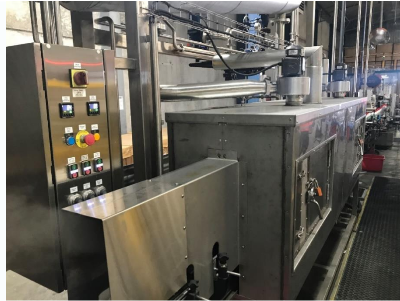
NEW sleeving tunnel in bleach plant
