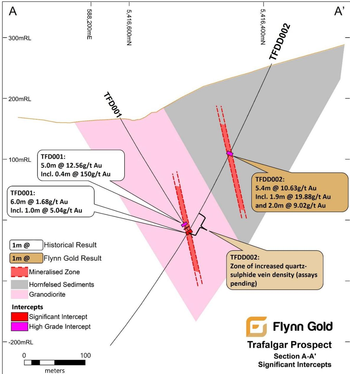
**Figure 3.** Cross-section A-A', Trafalgar prospect showing significant mineralised drill hole intercepts.
