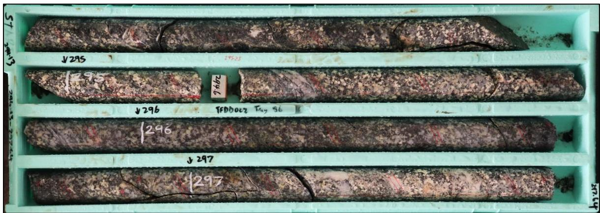
**Figure 8.** Example of TFDD002 core showing quartz-sulphide veining in altered granodiorite host rock, 294.1-297.6m.
