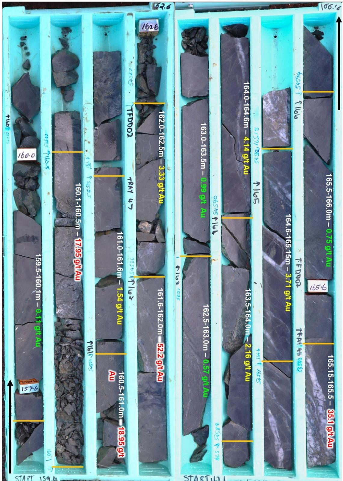
**Figure 4.** Photograph showing the selectively sampled TFDD002 core with sample intervals and assays, 159.4-166.15m.
