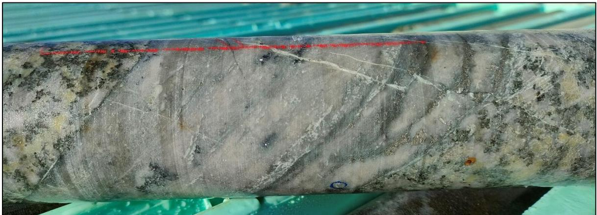
**Figure 9.** Example of TFDD002 core showing laminated quartz-sulphide veining in altered granodiorite host rock at 365.7m.
