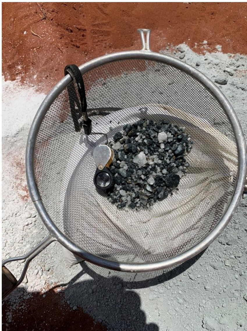
Plate 4: 21BRC0012 - Quartz carbonate veined mafic-ultramafic intrusive showing 3-5% disseminated sulphide (pyrite).
