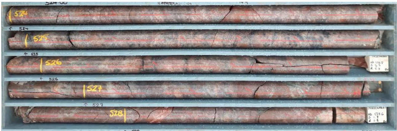
Figure 3: Sheared granite exhibiting zones of pervasive silicification, quartz veins, and some skarn development with minor K-Feldspar, albite, mica and actinolite alteration.
