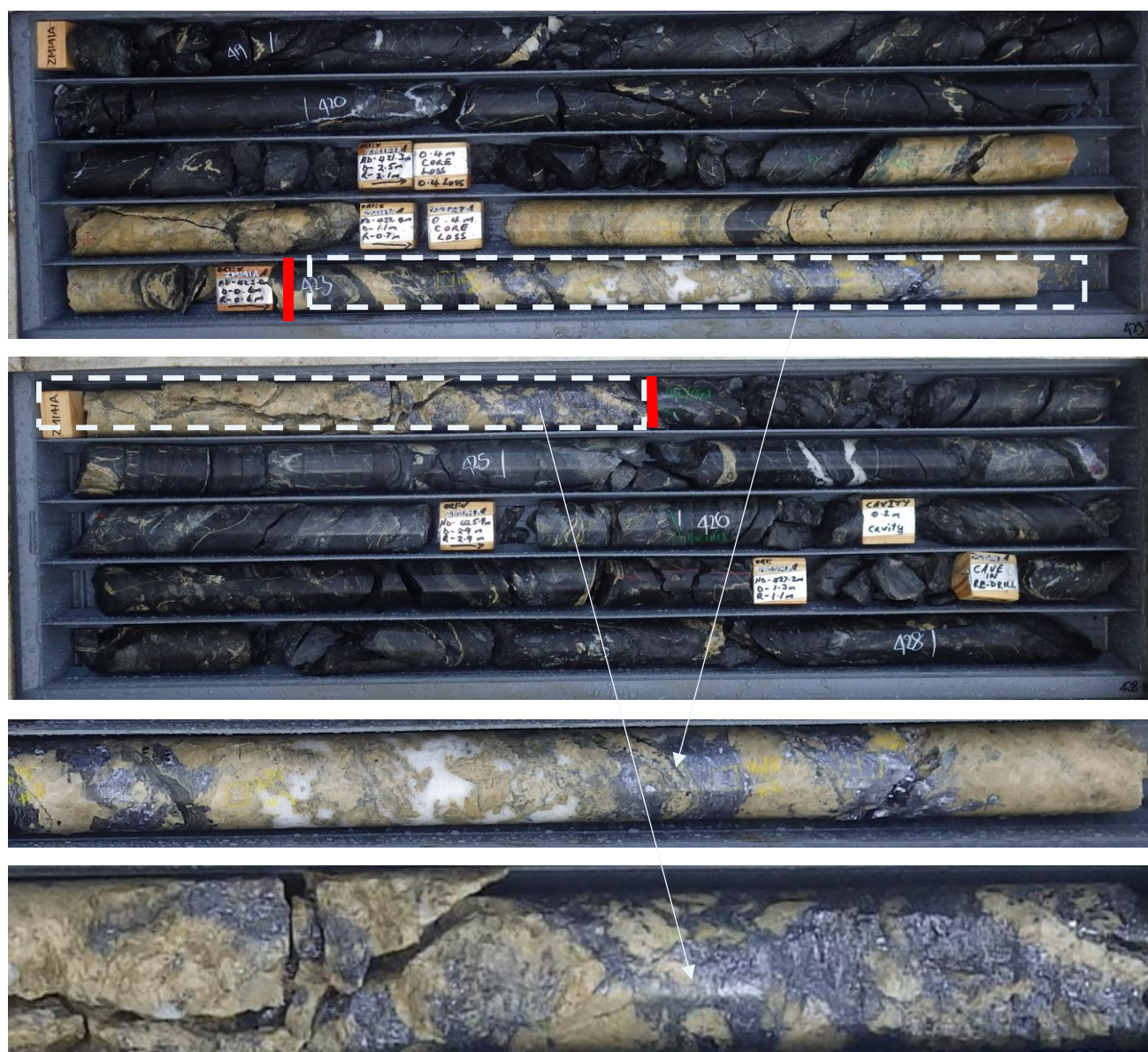
Figure 2 - ZM141A: Silver-Lead-Zinc mineralisation from 423m to 424.2m with visible galena and sphalerite
