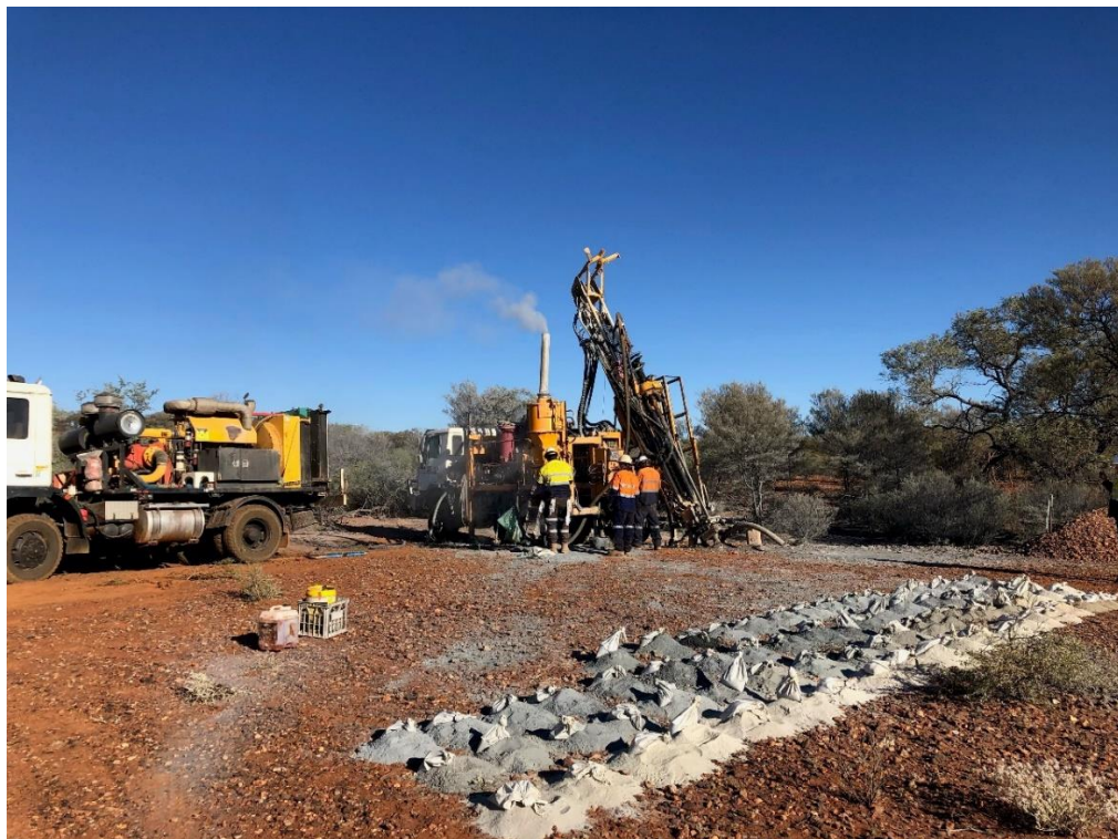
Figure 1. Impact Drilling air core rig set up and drilling the first hole at Green Rocks, testing geochemical anomalism.
