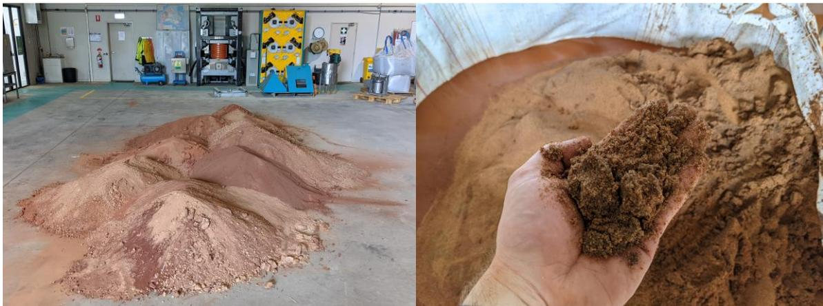
**Figure 2:** Bulk sample from Koko Massava deposit of 6.5 t pre-desliming and post desliming, work currently taking place by IHC Mining at their Metallurgical Test Facility, Yatala, Queensland.
