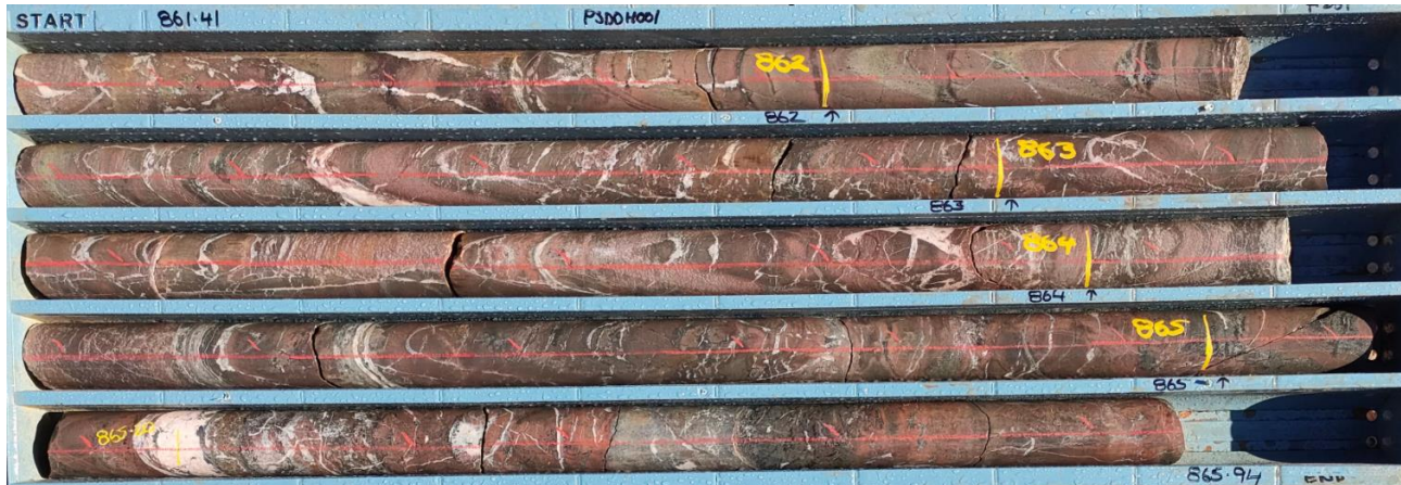
Figure 3: Drill core from PSDDH001 showing quartz-carbonate-hematite alteration with minor galena
