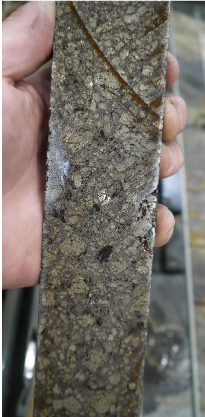
Figure Four | Image of Historic Drill Core from Kingsley meta-VMS deposit.
